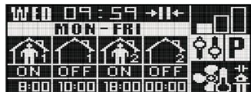
An example of the programmed calendar (working days). The device will be switched on at 8 a.m. and it will be switched off at 10 a.m. It will be switched on again at 6
